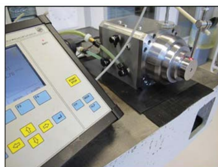
Fine tuning of balancing quality on the spindle
