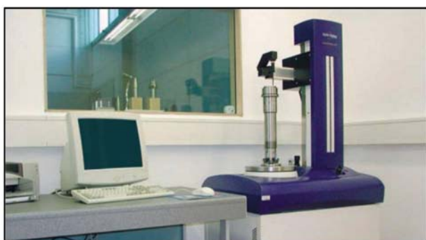
True-running gauging machine (to test rotation-symmetric parts of a spindle)
